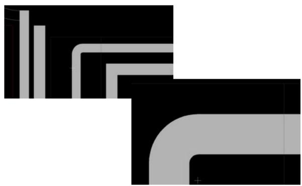
Below is an example of multiple traces drawn in different modes (like regular arcs, arc areas can be constructed using 8 different methods, although the default method is an arc tangent to the preceding segment, linear (solid) or arc (solid arc).
